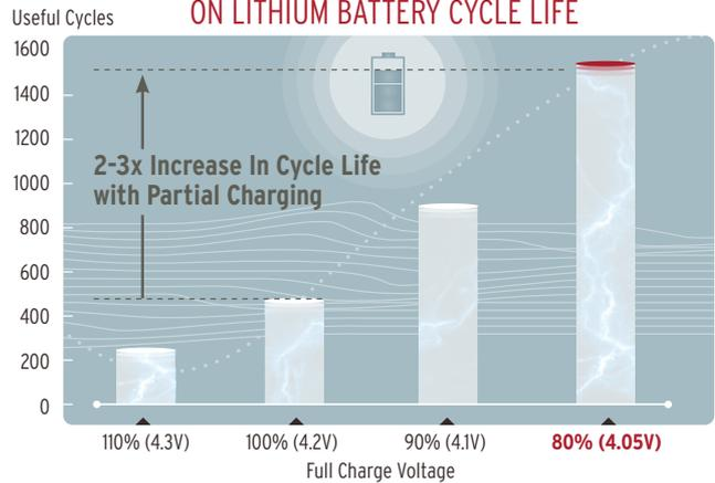
With the Cycle Satiator, you can program your primary profile to give an 80% charge, and have a secondary profile that does a 100% charge when you need full range. Then have the best of both worlds, a battery that lasts thousands of cycles but still goes the distance when you need it.
